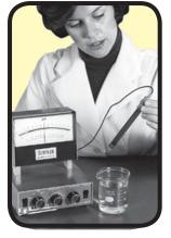
Model 140 is a 0 to 14 pH meter with 2 pH expanded scale and millivolt ranges. The 5.5" taut-band meter is in a tiltable housing for convenient viewing. Mirrored scale eliminates parallax problems and is readable to 0.01 pH or 2 mv. The plus and minus mv ranges are switchable with either plus or minus upscale. All controls are on the front panel. Temperature compensation is from 0°C to 100°C and a 10-turn calibration control enables the expanded scale to be set to any 2 pH range
